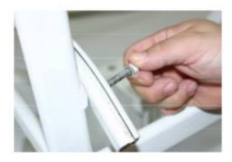
Step 4 - Insert Sling Spline
