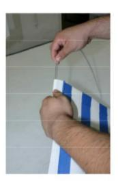
Step 5 - Insert Material Into the Sling Rails
