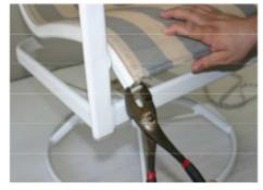
Step 2 - Remove the Old Sling Material
